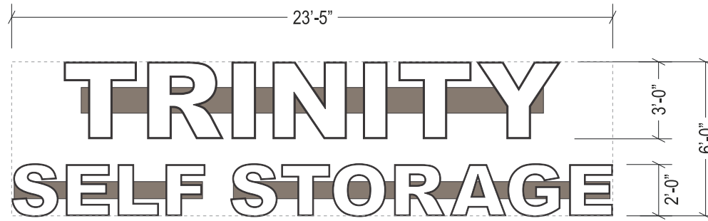
SIGN-A: LED ILLUMINATED PCL ON RACEWAY Scale: 3/16" = 1'-0"
