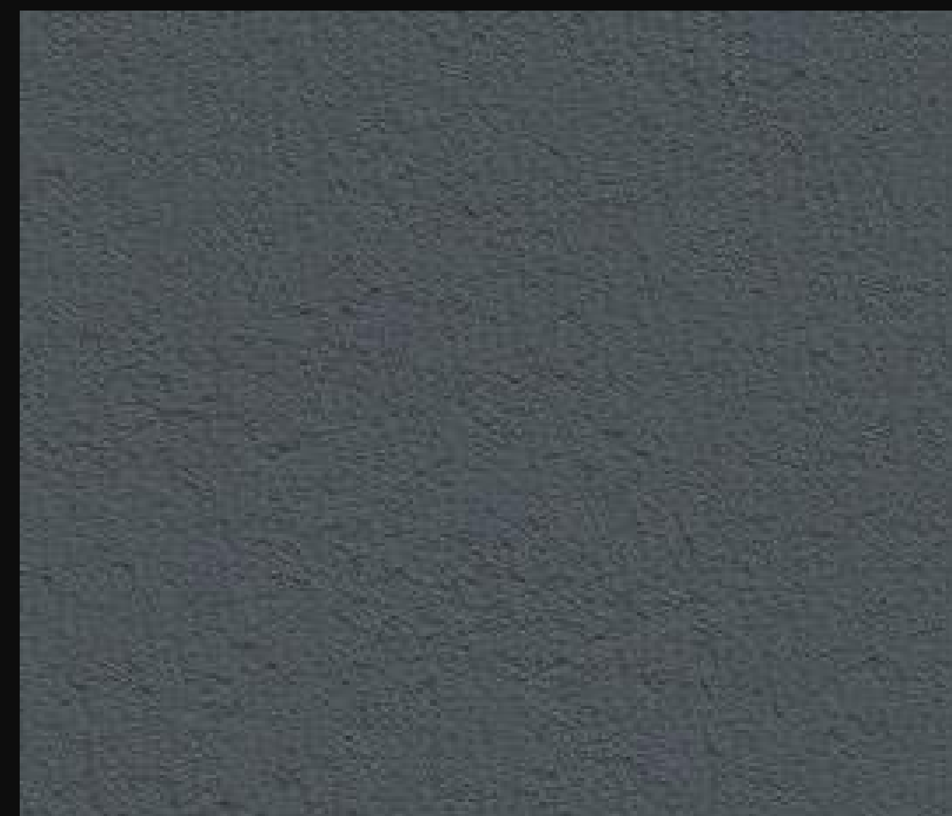
STUCCO SYSTEM MANUFACTURER: DRYVIT PROFILE: CCP-2 SYSTEM, SANDPEBBLE FINE E FINISH COLOR: PAINTED, BLDG DB GRAY DARK
