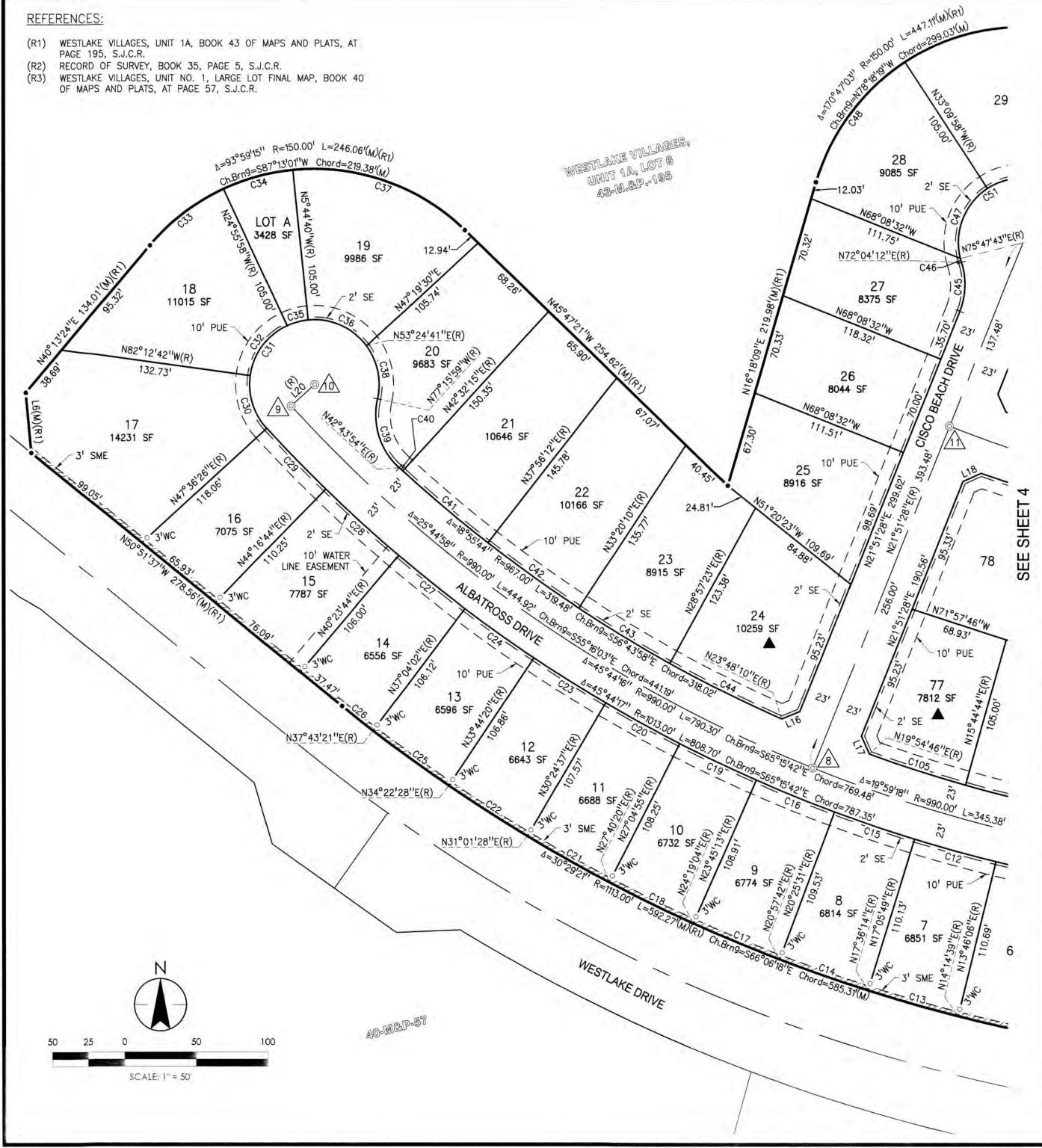
LINE DATA TABLE BEARING DISTANCE LINE L6 N5°11'07"W 42.12 L16 N67°45'11"E 13.68 L17 N24°02'15"W 13.68 L18 N65°43'57"E 13.97' L20 N47°36'26"E 22.001
