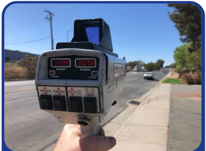
The ProLaser LiDAR device is used to detect vehicle speeds with an accuracy level of +/- 1 MPH.
