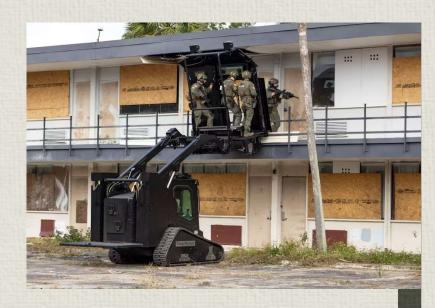
The "Rook" is an armored tracked vehicle. The protection and size of the vehicle allow for access to scenes not feasible by the Bearcat.
