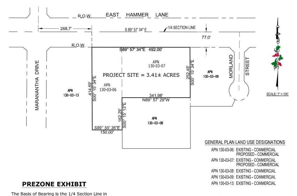
The Basis of Bearing is the 1/4 Section Line in Hammer Lane, which bears S 89° 57' 34" E per that survey filed in Record of Surveys, Volume 36, Page 195, San Joaquin County Records.
