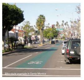
CLASS III BIKEWAY (BIKE ROUTE) MIXED-TRAFFIC CONDITIONS FOR BICYCLISTS USING SIGNAGE, STRIPING, AND/OR TRAFFIC CALMING TREATMENTS.
