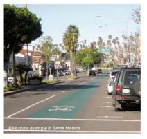
CLASS III BIKEWAY (BIKE ROUTE) MIXED-TRAFFIC CONDITIONS FOR BICYCUSTS USING SIGNAGE, STRIPING, AND/OR TRAFFIC CALMING TREATMENTS.
