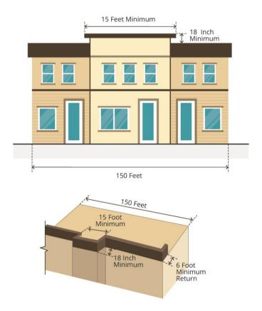
FIGURE 3-11D MIXED USE BUILDINGS, ROOF LINE
