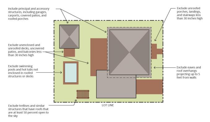
FIGURE 3-7 CALCULATING SITE COVERAGE
