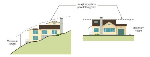
FIGURE 3-3 HEIGHT MEASUREMENT
