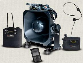
The LRAD is a specialized loudspeaker used for communicating at a distance, negotiations with barricaded suspects, mass notifications, and natural emergencies.
