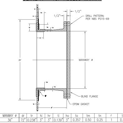
DRILL PATTERN: (PER NBS PS15-69) BOLT CIRCLE: 45"ø HOLES: (36) 7/16" -46<mark>3</mark>"øO.D.--42"øl.D. 37<del>1</del>"  $27\frac{1}{2}$ " -90"øl.D.--96"øO.D.-
